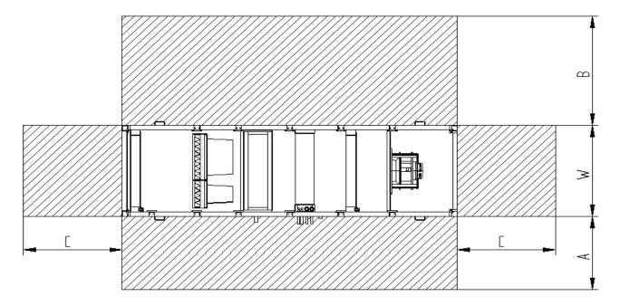
The unit must be put in a position where there is sufficient space for performing routine and extraordinary maintenance. Observe the following points:
