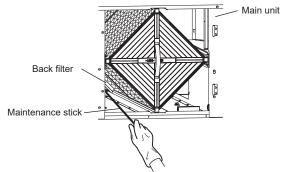
3. Hold the handle and draw the Lossnay cores out from the main unit.
