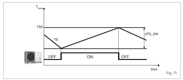
DHW is requested when T5S - T5  $\geq$  dT5\_ON
