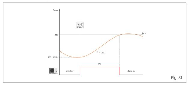
This value is strongly related to the minimum permissible water content of the circuit. A narrower control band can be accepted with a high water volume.
