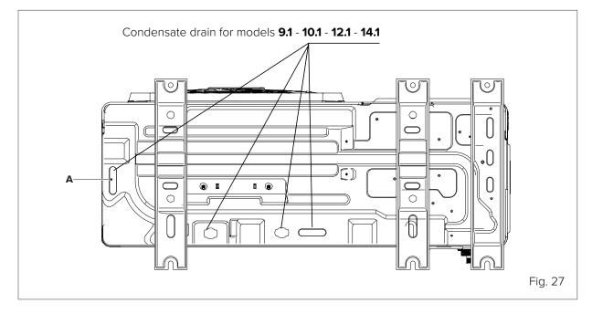
The drain hole (A) is covered by a rubber plug. If the smaller drain hole cannot fulfil the drainage requirements, the larger drain hole can be used at the same time.
