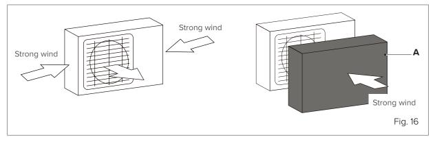
If the wind direction can be predicted, refer to the figures below for installation of the unit. Turn the air outlet side towards the wall, boundary element or building shield.
