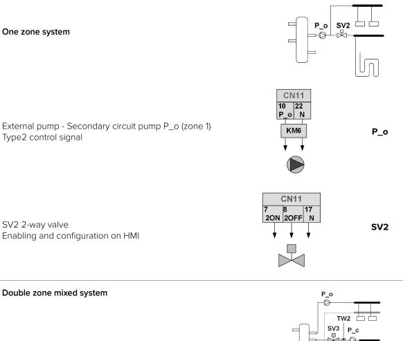
External pump - Secondary circuit pump P\_o (zone 1) Type2 control signal
