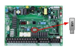
With the unit powered and switched **Off** plug the flash drive into the USB port on the indoor unit board.
