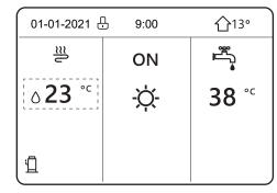
Press any button: the UNLOCK icon will flash. Long press the UNLOCK button ( ). The icon will disappear from the screen and the interface can be checked.
