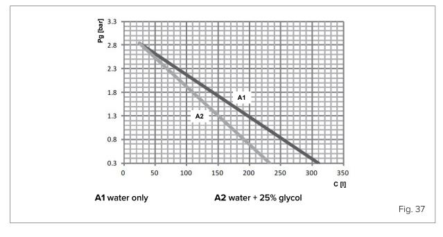
The total volume of water in the system must be less than that indicated, otherwise an additional expansion tank will be required.
