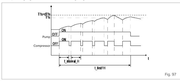
The operating logic is shown in the following diagram:
