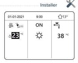
Double zone system 01-01-2021 9:00 **1**3° • Keypad control: MENU > FOR SERVICEMAN > ROOM THERMOSTAT > ≝ ON **ROOM THERMOSTAT= NON** Press the back button ٥23 ٥C -Ò-Select temperature type settings > double zone = yes °C 38 • Thermostat control:
