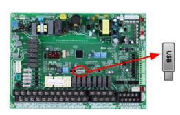
With the unit powered and switched **Off,** plug the flash drive into the USB port on the indoor unit board.
