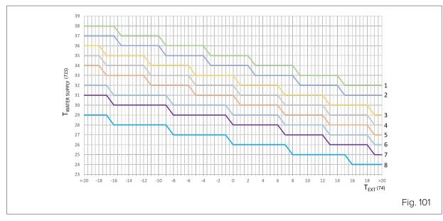
• 8 default curves for Heating mode on systems with radiant distribution.
