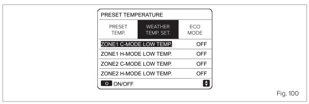
During the year, the heat load of the building is highly variable depending on factors such as outdoor air temperature, insulation, thermal inertia, crowding, etc. So in Heating mode, it is advisable to use the setpoint setting on the automatically controlled water supply or on the indoor air (which controls the water supply with the climate curve).
