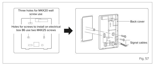
Prevent water from entering the wired controller, use siphons and mastic to seal the wire connectors during installation.
